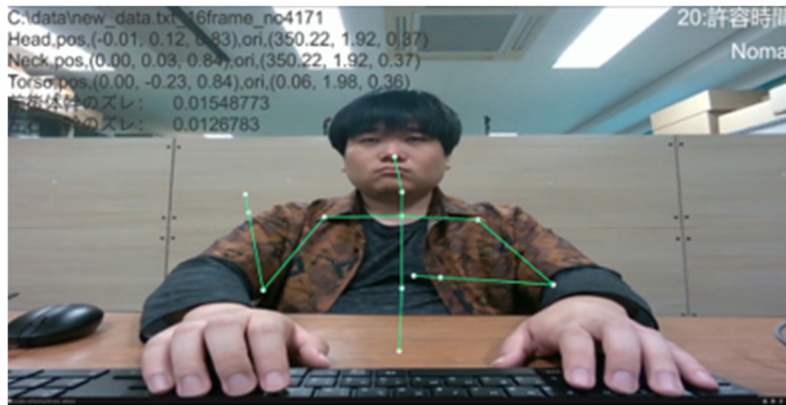
Fig. 3. Body tracking from a depth-camera
